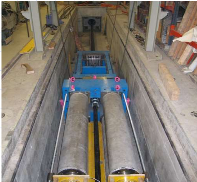
Fig. 2 Servo-hydraulic jack with a 43-strand stay cable anchorage
