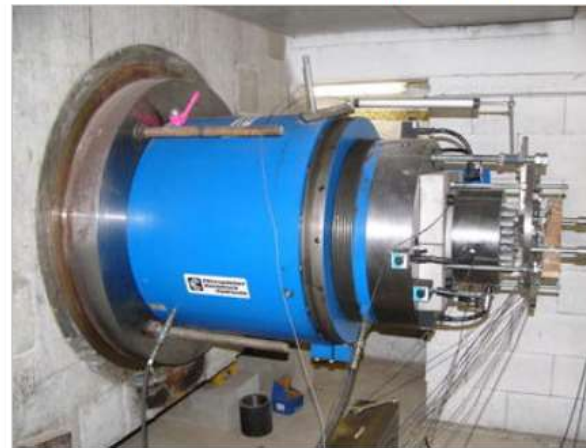
Fig. 2 Servo-hydraulic jack with a 43-strand stay cable anchorage
